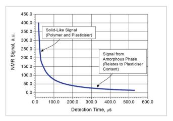
**Figure 1:** Typical NMR signal from polymer
